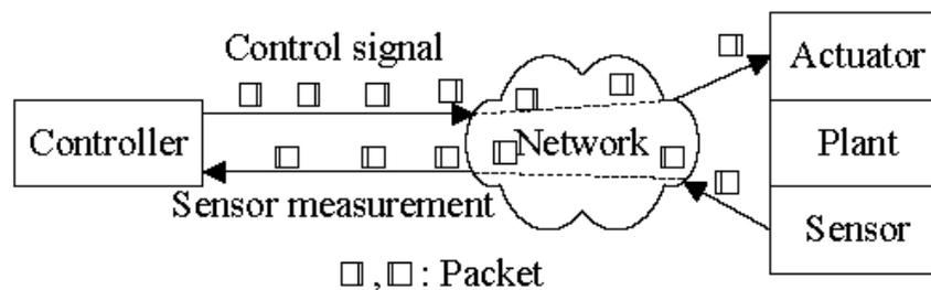
Figure 1. Direct structure of networked control system.
