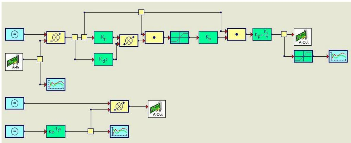
Figure 5. MCON implementation of control system with quasi-relay variable structure-PI controller
