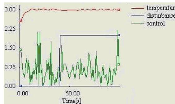
Figure 7. Controlled temperature (red), disturbance input (blue) and control signal (green) versus time for control system with de-tuned controller parameters.
