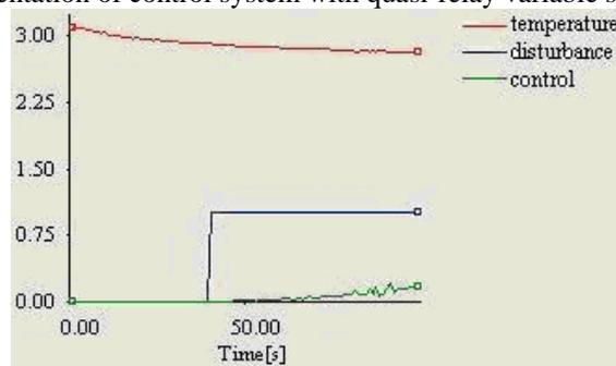
Figure 6. Controlled temperature (red), disturbance input (blue) and control signal (green) versus time.
