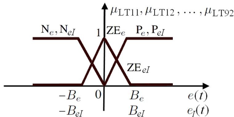
Figure 3. Input membership functions of Takagi-Sugeno-Kang Proportional-Integral fuzzy controller.
